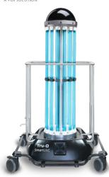
The **Tru-D**® robot is a portable UV disinfection system that delivers an automated, measured dose of UVC to consistently disinfect a room in a single cycle, resulting in the ability to document disinfection results after each and every **Tru-D** room treatment.
